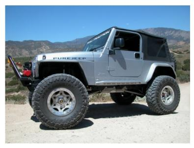
This instruction sheet will cover the installation of our standard TJ rockers as well as the sheared version for use with our PJ4000 Tube Fenders. Included are a pair of rockers, hardware to mount the rocker to the side of the Jeep as well as spacer pucks and hardware to mount through the tub as well.
